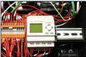
**Programmable Smart Control Automation** provides complete control over the machine's run time, auto start/stop and time delay shut down functionality.
